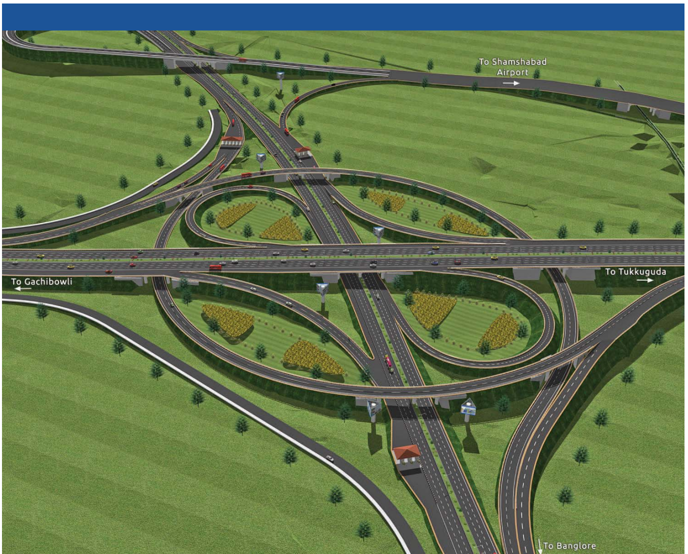
A partial Clover Leaf interchange on the expressway
